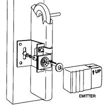
Keeping the sensors pointing in towards door and aimed at each other, tighten nut until there is enough friction to hold in place. Do not fully tighten until the final alignment has been completed.
